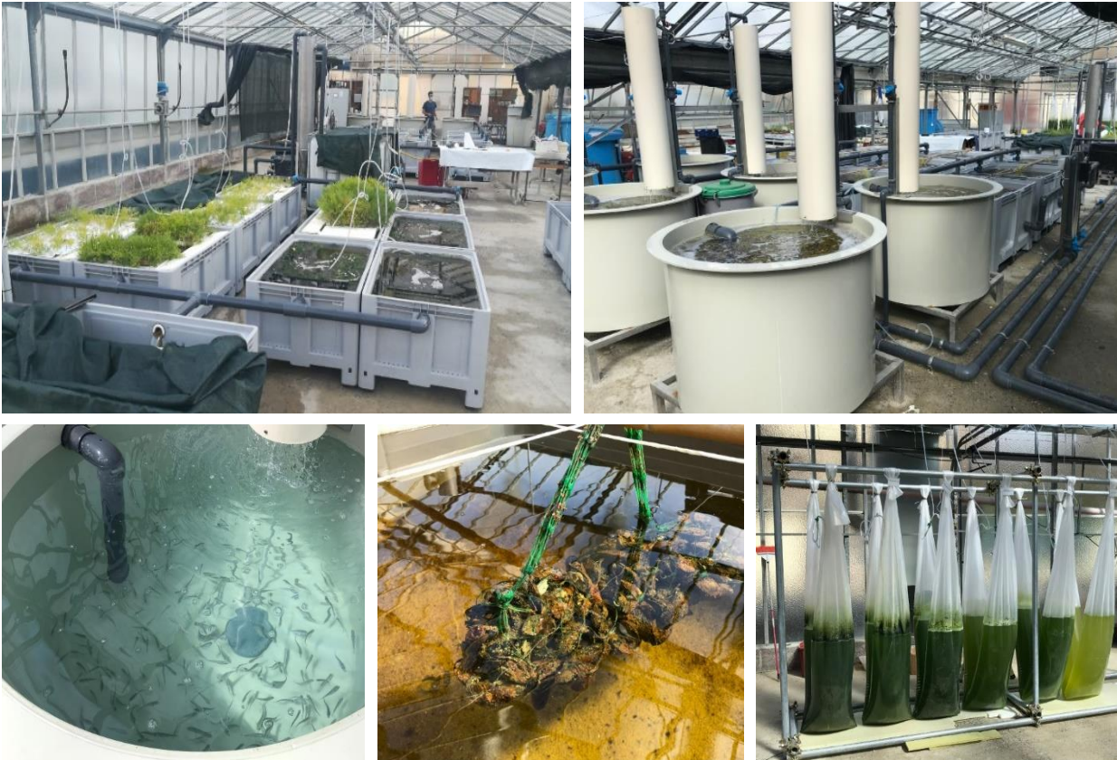
Fig. 2. Some views of the SIMTAP system installed at the University of Pisa. From left to right, top to down, sections for seaweeds and halophytes ( Salicornia europaea L.), fish, DFFO (mussel Mytilus galloprovincialis ) and photobioreactors with microalgae (SEC_LI_ChL_1 strain and Chlorella sorochiniana ).
