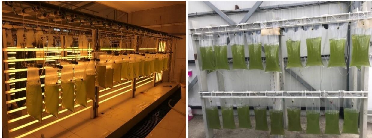
Fig. 25. The photobioreactors used at the Mediterranean Fisheries Production and Training Institute (MEDFRI), Antalya, Türkiye for the experiments with Tetraselmis suecica culture in marine aquaculture wastewater in the laboratory or in greenhouse.
