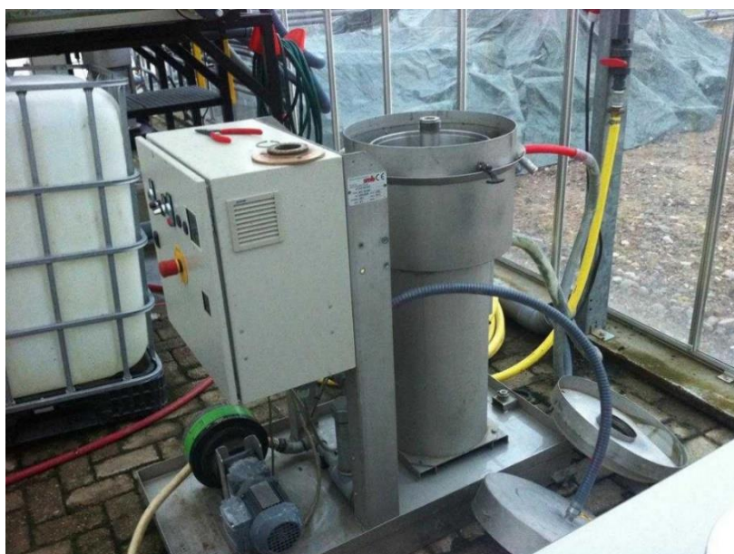
Fig. 26. A centrifuge to harvest microalgae biomass.
